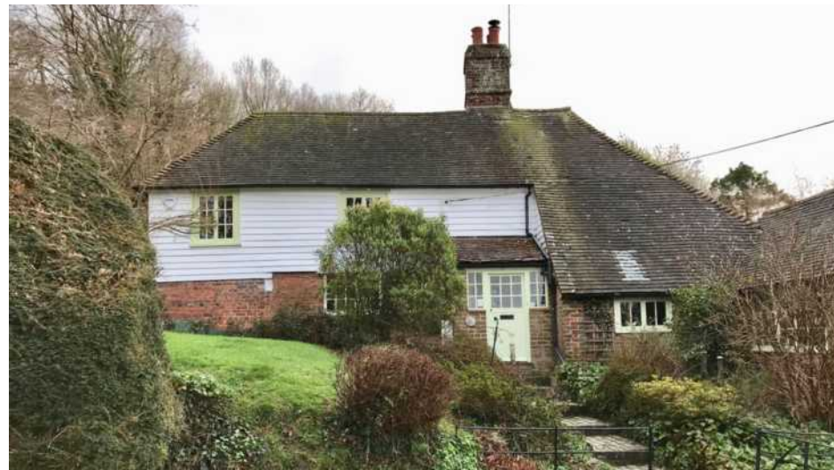
Above: Many of the older cottages have a brick ground storey and timber clad upper storey as in this example on Sampson's Lane. Image credit: Deeper Green
